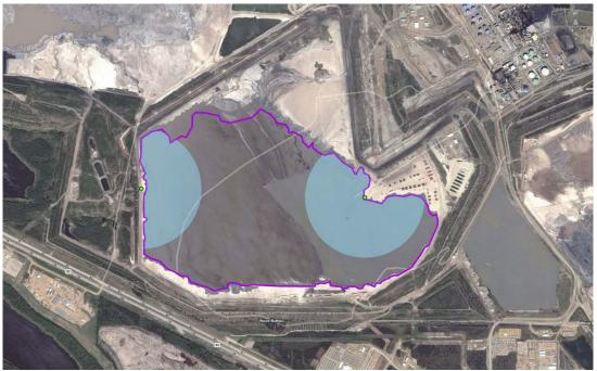
Figure 5.1. Example of survey station positioning at Suncor pond 2/3. Pond surface area is approximately 2.7 km<sup>2</sup> and circles illustrate 500m radius from survey station.
