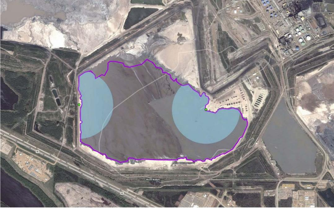
*Figure 5.1. Example of survey station positioning at Suncor pond 2/3. Pond surface area is approximately 2.7 km<sup>2</sup> and circles illustrate 500m radius from survey station.*
